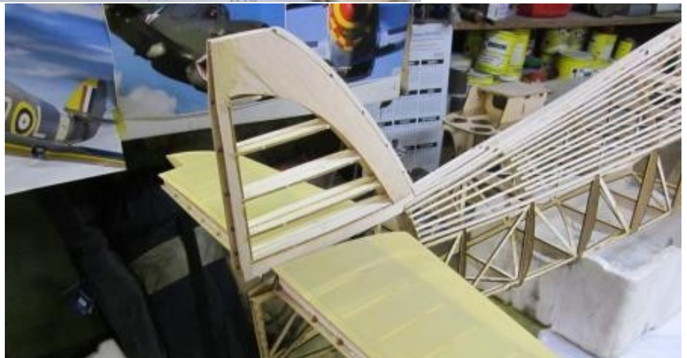
This picture shows the fin perched over the void at the rear end of the fuselage frame.
