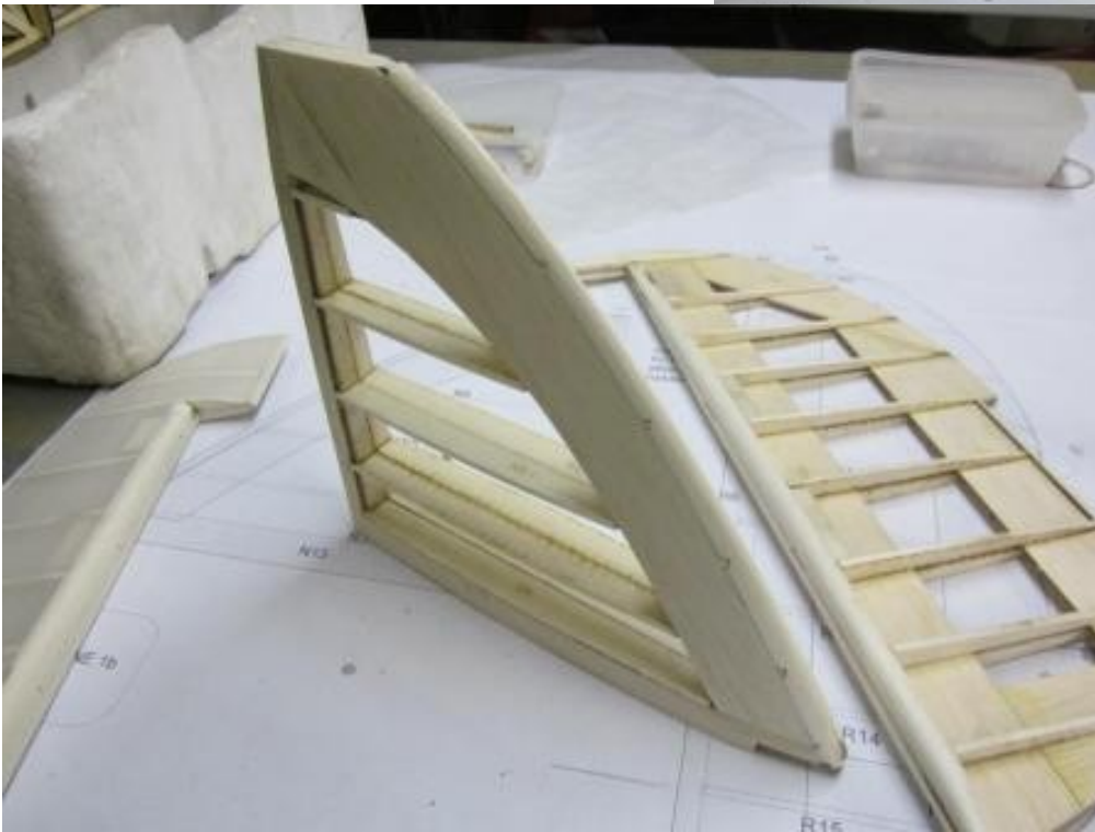
Finished fin and rudder ready for covering.
